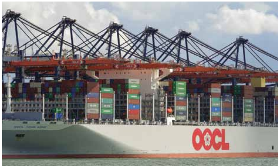
The world's largest container ship as of 2017, the OOCL Hong Kong has a capacity of 21,413 twenty-foot equivalent units. Its Wartsila-Sulzer RTA96-C engine runs on bunker fuel.
